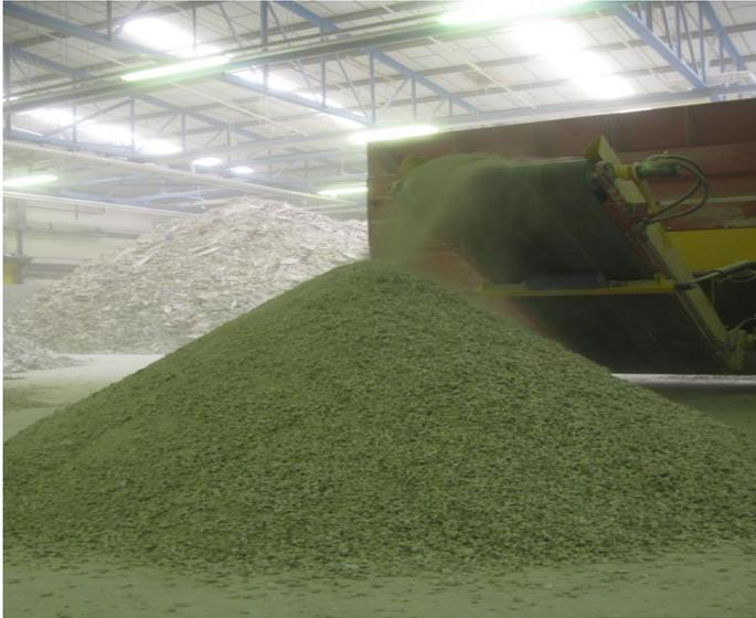
First part of the recycling process is to remove any contaminants and grind the material into small pieces.
